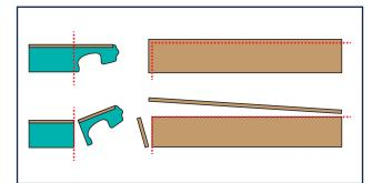
3. To achieve a perfect fit, always fit a cut edge next to walls rather than a locking profile. For pieces that sit in the corner of a room, this will mean cutting both the long and short edges to remove the locking profile.
