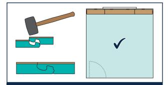
5. To install the first row, align the short edge joints and gently tap into place using a soft rubber mallet. Be sure to align the joints accurately and tap directly in line with the joint to ensure a perfect seal. Continue to install further pieces until the first row is complete.
