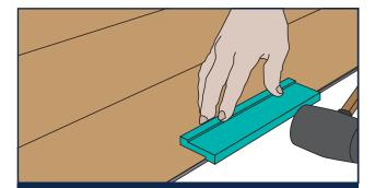
7. Continue to lay pieces along the second row by locking the long sides to the previous row. Gently tap the short edge joints with a soft rubber mallet to secure into place. Use a soft rubber mallet and a tapping block to make sure all joints are locked flush to one another.
