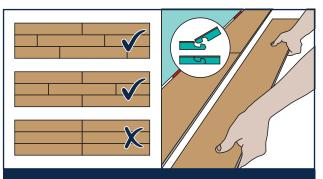
6. To attach the long edges, insert the tongue side into the groove side of the previous piece at an angle of around 30°. Gently apply inwards and downwards pressure until the joint closes and the pieces lay flat. Always ensure the joints are staggered by at least a third.
