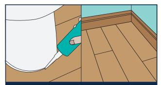
9. Continue to work left to right row by row. Once the floor is complete, remove the spacer wedges. Finish the look with skirting boards around the perimeter to conceal the expansion gaps. For splash areas such as bathrooms, high quality silicone caulking should be used to prevent water seepage.
