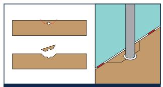
8. ClickLux can be easily fit around pipes by using a hole saw. Use a utility knife and cut a few centimeters away from the hole horizontally then at a 45° angle to the edge. Always leave a 6mm expansion gap around all pipes and objects. Reattach the pieces together using PVA glue and wipe away any excess glue with a damp cloth.
