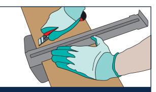
2. To cut your ClickLux planks to size, measure and mark with a pencil. Using a T-square and utility knife, apply pressure and score along the line. Gently flex along the scored edge until it separates into two pieces.
