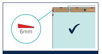
4. Begin installing ClickLux from the left side of your room and always work to the right. Use spacer wedges next to any piece that meets a wall to ensure a 6mm expansion gap is left around the perimeter.
