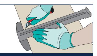
2. To cut your ClickLux tiles to size, measure and mark with a pencil. Using a T-square and utility knife, apply pressure and score along the line. Gently flex along the scored edge until it separates into two pieces.
