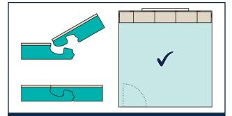
5. To install the first row, insert the tongue side into the groove side of the previous piece at an angle of around 30°. Gently apply inwards and downwards pressure until the joint closes and the pieces lay flat. Continue to install further pieces until the first row is complete.
