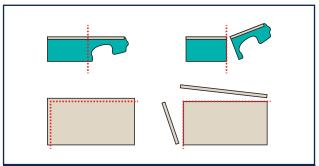
3. To achieve a perfect fit, always fit a cut edge next to walls rather than a locking profile. For pieces that sit in the corner of a room, this will mean cutting both the long and short edges to remove the locking profile.
