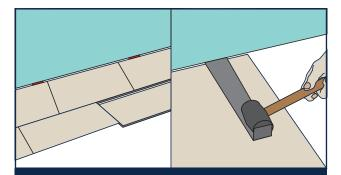
7. Continue to lay tiles along the row. Always connect the short edge first, then lift and angle the long edge into place. As you angle the long edge, the previous tile will lift at the same time. Use a pull bar at the end of a row to ensure the joints are secured.
