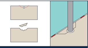
8. ClickLux can be easily fit around pipes by using a hole saw. Use a utility knife and cut a few centimeters away from the hole horizontally then at a 45° angle to the edge. Always leave a 6mm expansion gap around all pipes and objects. Reattach the pieces together using PVA glue and wipe away any excess glue with a damp cloth.
