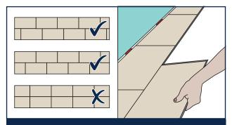
6. When starting a new row, always remember to work from left to right. Pieces can be easily locked together on the long edge by angling the joint and applying pressure in the same way as the short edge. Always ensure the joints are staggered by at least a third.
